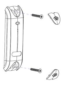
Screw unit to the surface. Place caps on to the unit and push firmly into place.
